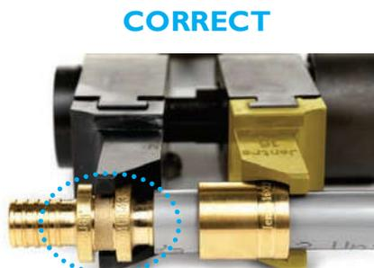
▲ Fig. 38: Black clamping head placed correctly.
