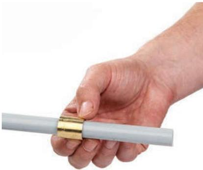
▲ Fig. 21: Push the compression sleeve over the pipe. The inside chamfer has to point to the end of the pipe.
