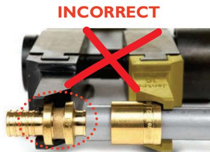
▲ Fig. 37: Black clamping head placed incorrectly.
