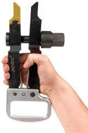
▲ Fig. 24: Caution: the clamping head behind the sleeve has a yellow chromed colour; use behind the flange edge the head with black colour!
