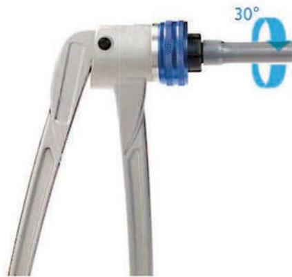
▲ Fig. 33: Expand PEX pipe.
