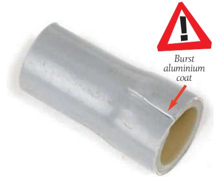
▲ Fig. 20: Cut the bad part completely away in a square angle and start over!
